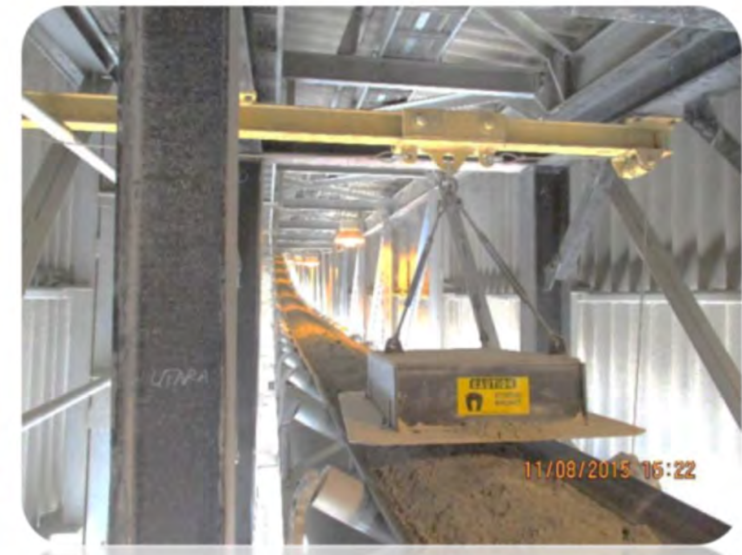
Stationary Permanent Magnet Type 13PCM36 PT. Semen Indonesia, Tuban East Java Year 2015
