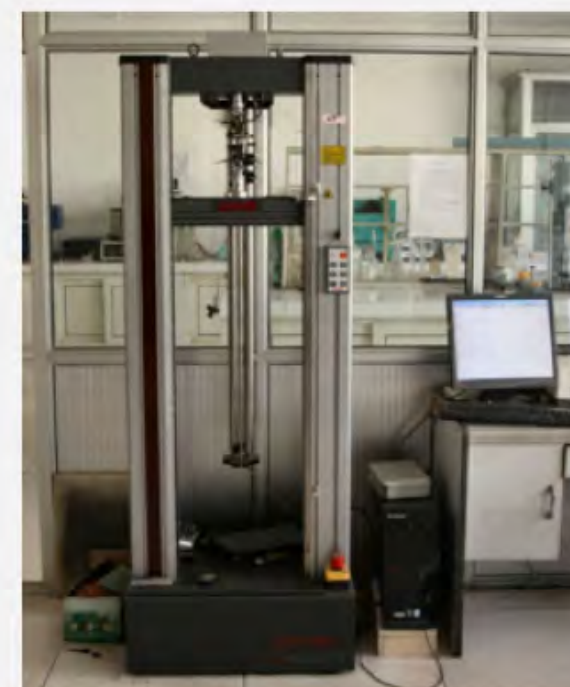
Tensile, tear, elongation, Testing
