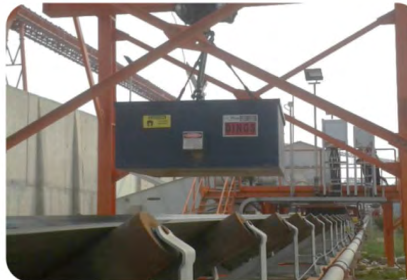
Stationary Electromagnetic PT. Suprabari Mapanindo Mineral Muara Teweh, Central Kalimantan Year 2015
